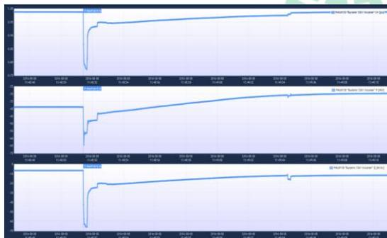
Figure 2-Load Dynamics & Voltage Recovery Performance at Buraimi substation
